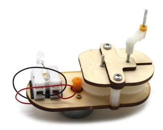
This hand-crank generator is an excellent STEM kit to demonstrate the transfer of mechanical energy into electrical energy. It is a compact device designed to convert mechanical power into electrical power. As students turn the crank, they directly power a small light bulb without the need for batteries. It's a hands-on way to illustrate the conversion of energy from one form to another.
