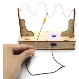
The Electric Conductivity Kit is an exciting STEM project that explores electrical conductivity, circuits, and the relationship between electricity, sound, and light. This kit is similar to the old game "Operation," where the goal is to avoid contact between the metal horn nail on the shaft and the conductive iron wire. When contact occurs, the circuit is completed, causing the LED light to illuminate and the buzzer to sound, demonstrating the principles of closed and open circuits.
